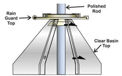
Drop joined Basin Top and Rain Guard Top into the slotted base.
